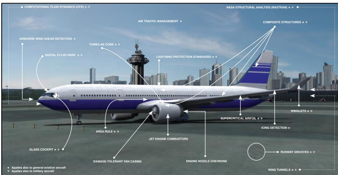
**Figure 7. Applications of NASA research results in a modern commercial airliner (illustrative).** Source: The European House - Ambrosetti elaboration on NASA, 2017
